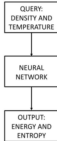
**Figure 1** (left): Diagram of model 1, a simple neural network design to model equations of state.
